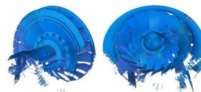
Figure 4. Runner of a hydroelectric power plant resulting from 3D scanning
