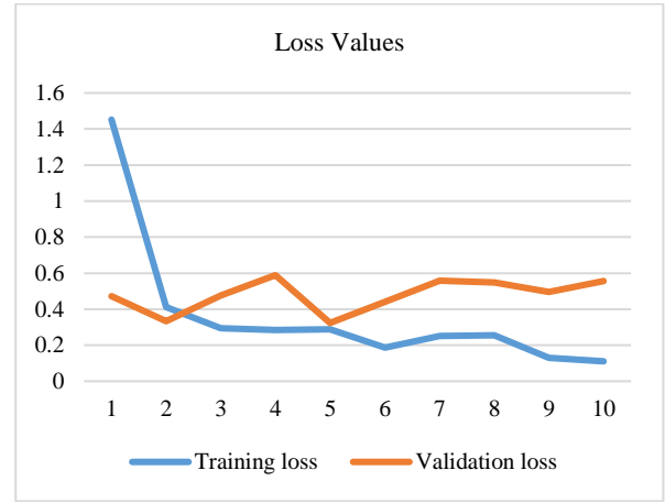
Figure 6. Train and val. loss in ViT 16x16
