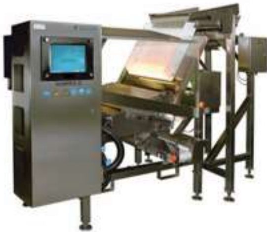
Figure 2. Optical sorting machine for sorting wet products ( https://www.refrigeratedfrozenfood.com )
