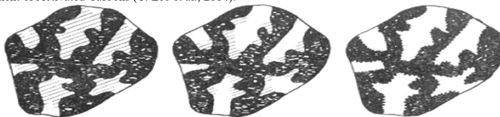
Figure 5. Gradual activation process of carbon during thermal treatment (Yahya et al., 2015b).
